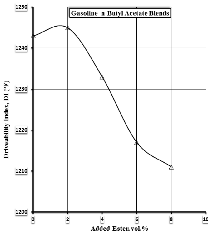
Fig. 10. Effect of n-Butyl Acetate Addition on Drivability Index of Fuel Blends
