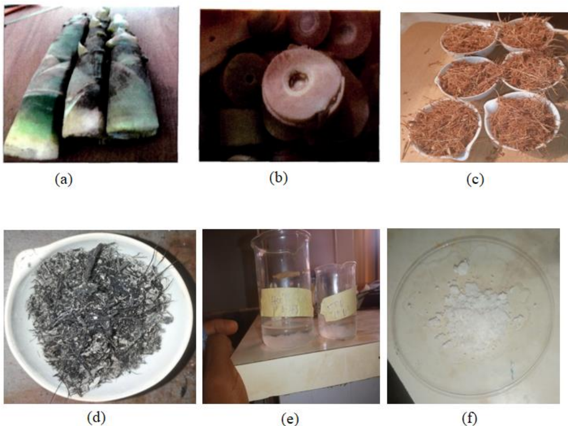
Fig. 1. Plates (a) Raw bamboo shoots (b) Cleaned and sliced bamboo shoots (c) Pounded and dried bamboo shoot (d) BSA (e) Crystal formation (f) Extracted silica gel
