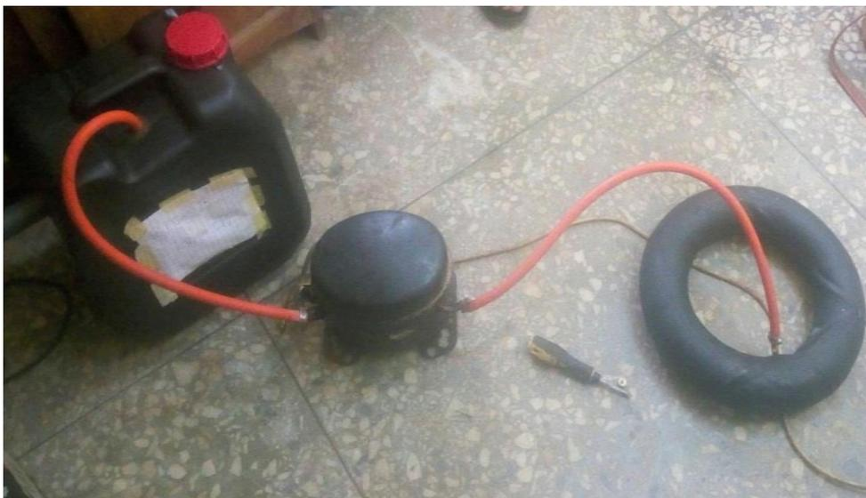
**Figure 2:** Set up of the fittings of the laboratory scale digester with compressor
